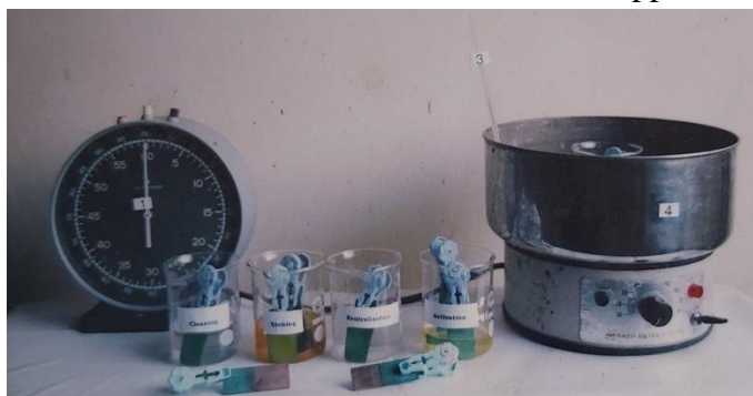
Fig. 1. Assembled equipment for the whole electroless copper plating process.
