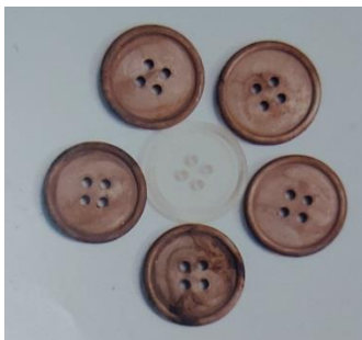
Fig. 5. Electroless plating of copper on plastic button.
