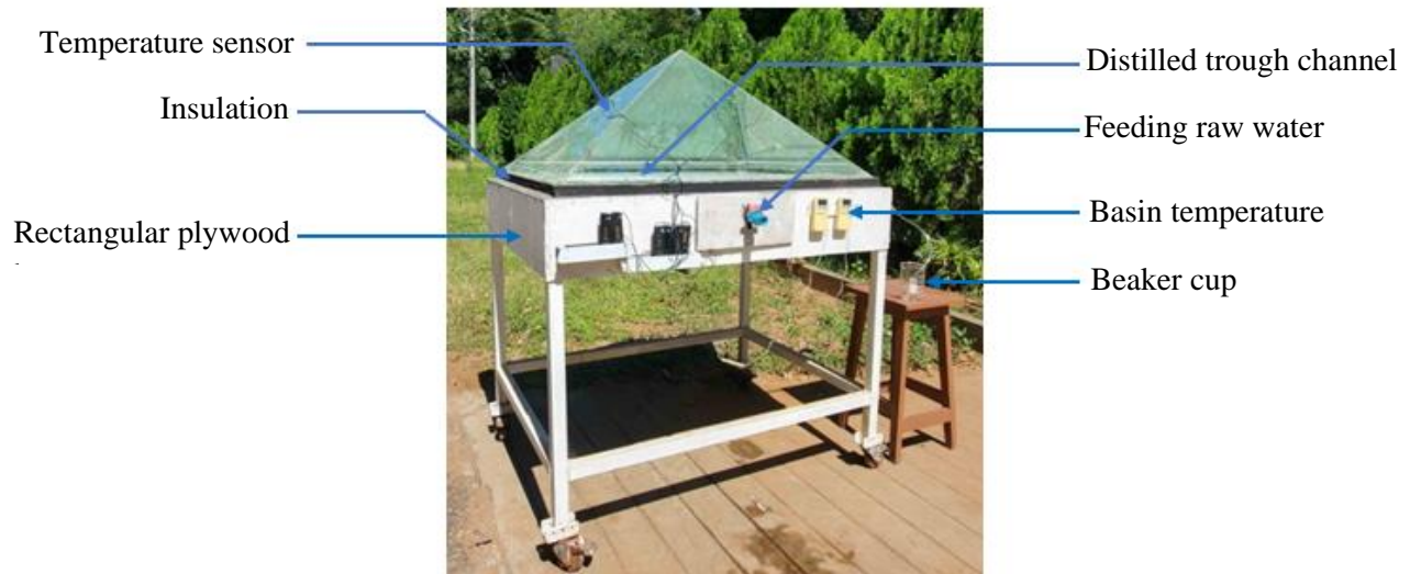
Figure 3. Experimental setup of pyramid solar still
