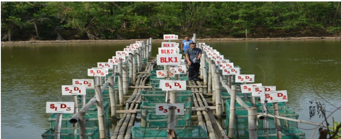
Figure 1. The Experimental Set up (S- Size of Cage; D-Depth of Embedding)
