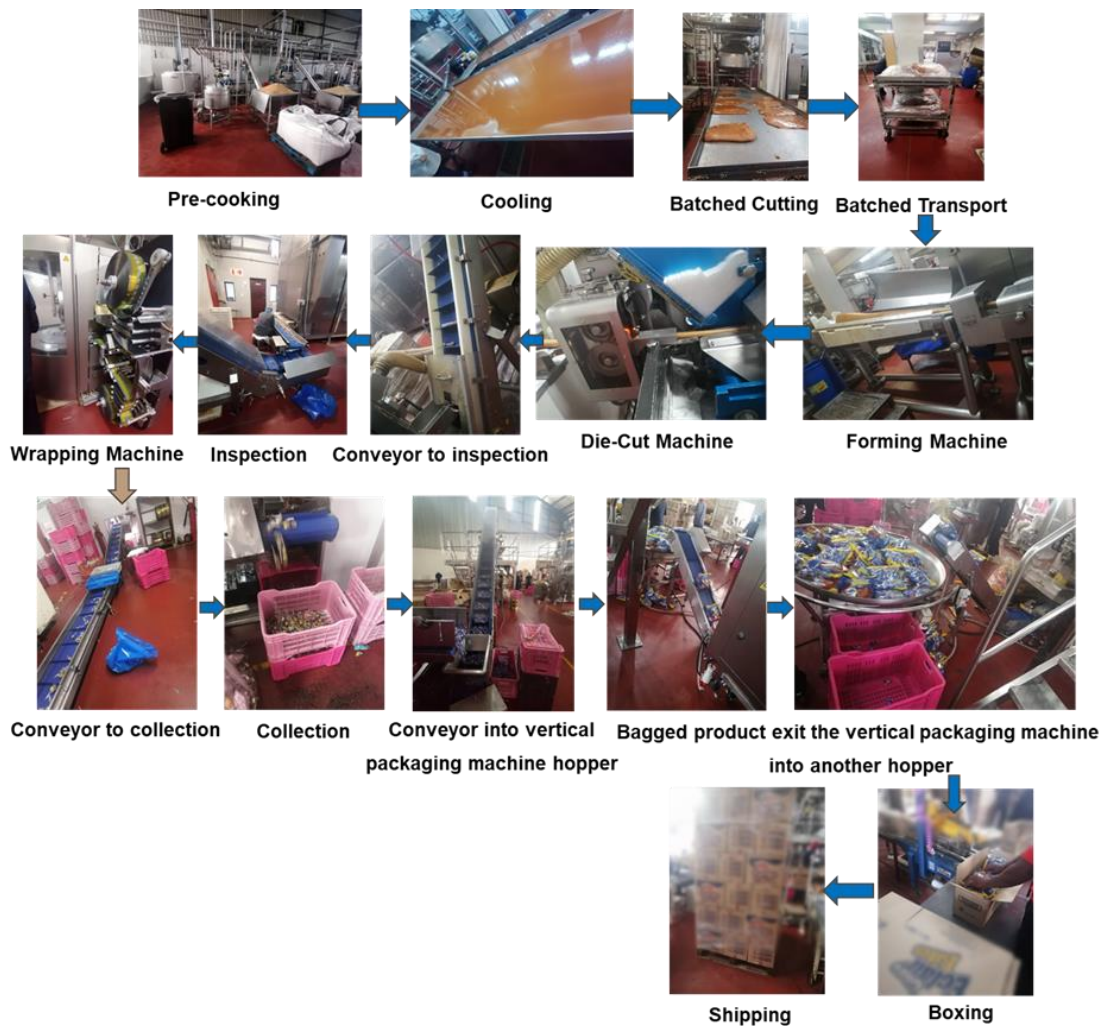
Fig. 3. Sequence of sweet manufacturing processes and tasks in the present case.
